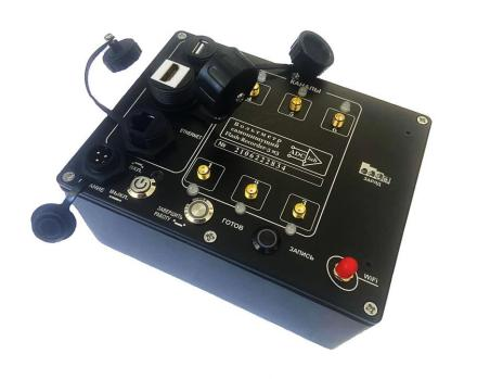
**Flash-Recorder-3** M4 — is high-speed version of the product line. The main feature is built-in ICP power supply for channels with 3 MHz sampling rate. 10000 mAh battery allows you to use the device distantly up to 8 hours of continuous operation.
